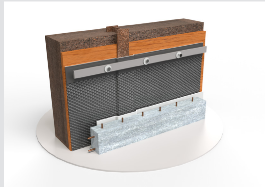
DELTA®-TERMINATION BAR fastened every 8" with nails.
