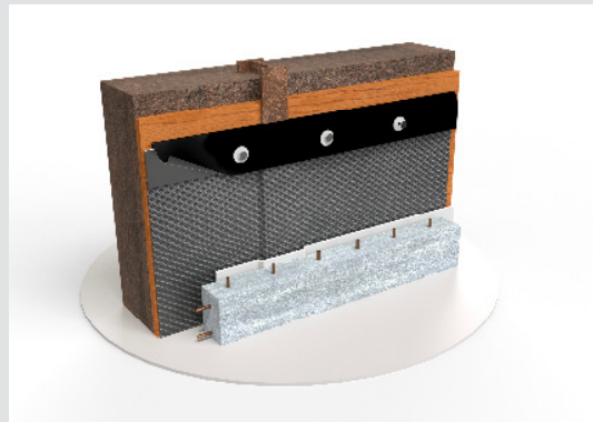
Nails with 2.25" washers placed along the flat tab every 8" on center.
