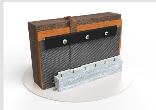
DELTA®-MOLD STRIP or DELTA®-FLASH fastened every 8" with nails.
