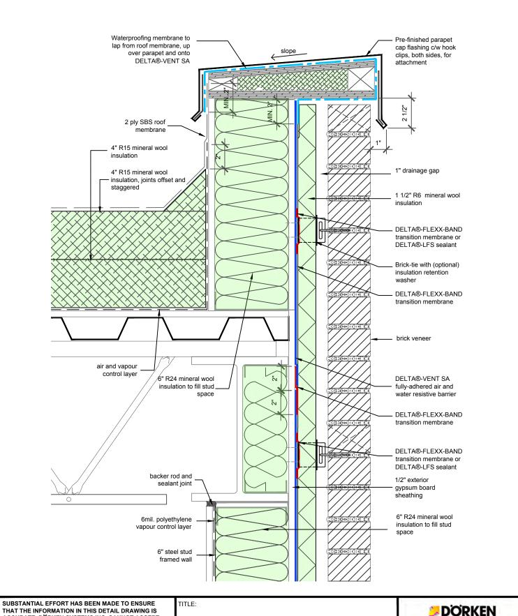
WALL ASSEMBLY #3: TYPICAL ROOF TO WALL **SECTION**
